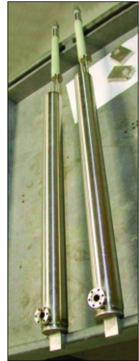
aPhoto of actual leads modeled on left with removable upper tabs detached
