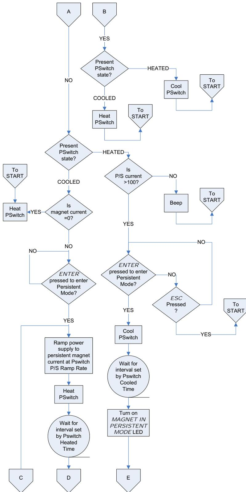
Figure A-15. Persistent Switch Operation Flowchart, Page 2
