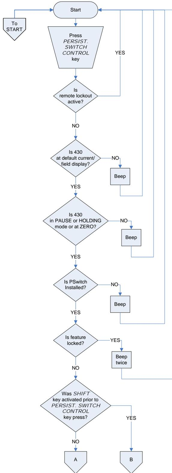
Figure A-14. Persistent Switch Operation Flowchart, Page 1
