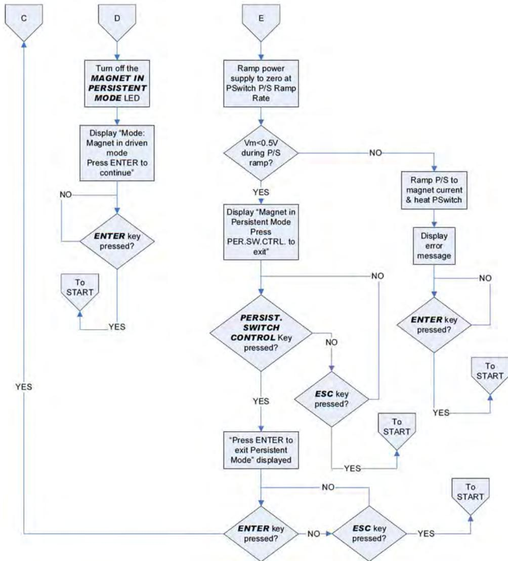
Figure A-16. Persistent Switch Operation Flowchart, Page 3
