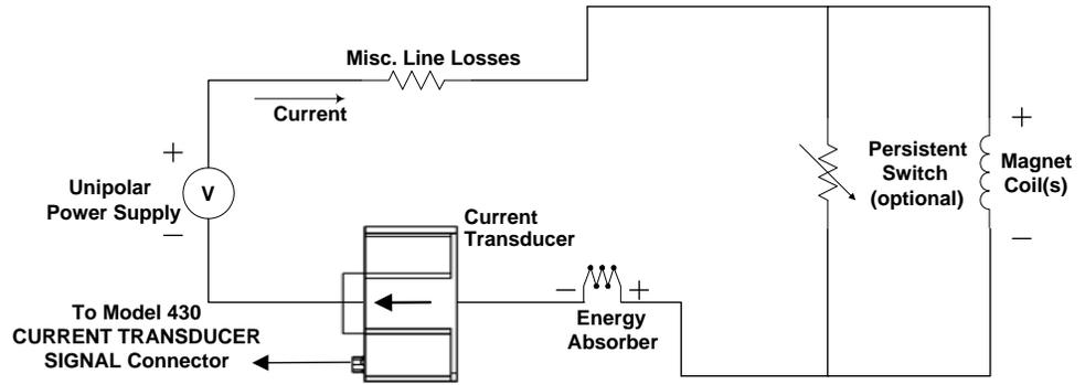
Figure 1-6. Dual-Quadrant System with Precision Current Transducer Option
