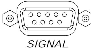
The current transducer signal connector provides pins for connection of the current transducer (CT) signal to the Model 430; power to the CT is also provided via this connector. The connector is a 9-pin D-sub female connector with the shell lugs connected to the Model 430 Programmer chassis ground.
