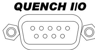
The Quench I/O connector provides pins for external quench detection input, quench detection output, and external rampdown input. The shell lugs of the connector are connected to the Model 430 Programmer chassis ground. The Quench I/O connector is a 9-pin D-sub female connector.
