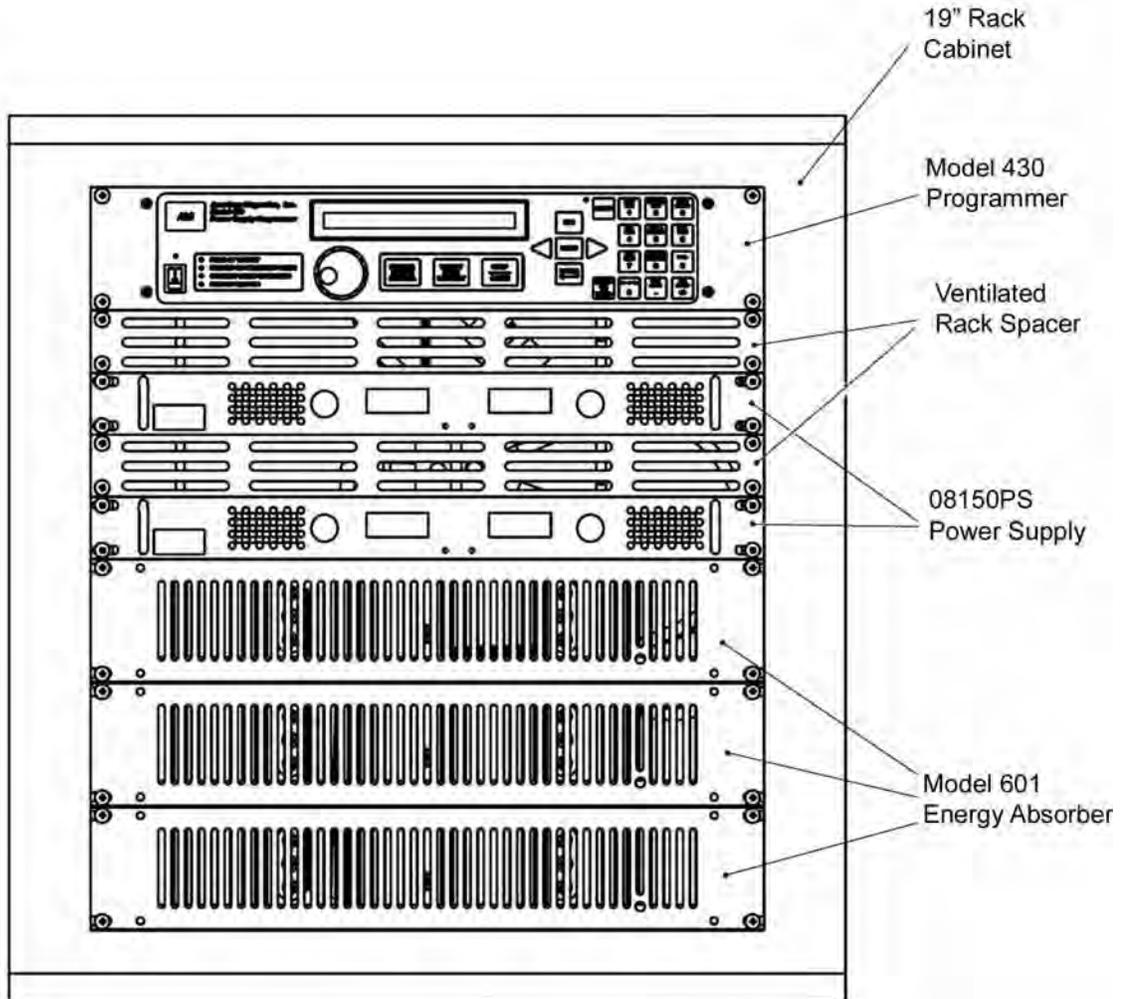
Figure 1-1. Typical Model 03300PS-430-601 System Rack Layout
