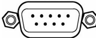
The RS-232 connector is a standard DTE 9-pin D-sub male connector
