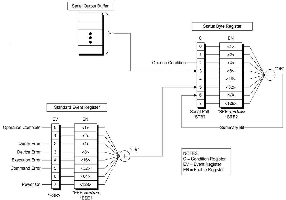
Figure 4-1. The Model 430 Programmer Status System.
