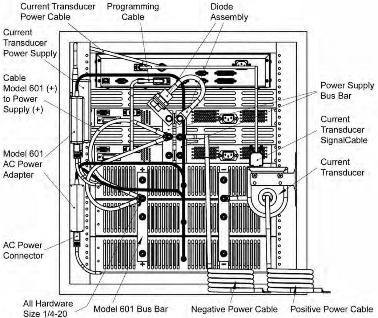
Figure 2-1. Typical Model 03300PS-430-601 System Rack Interconnections
