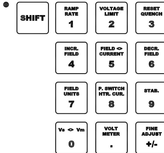
Figure 3-5. SHIFT-Key Functions
