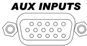
The Aux Inputs connector provides pins for external voltage inputs, reserved for future use. The shell lugs of the connector are connected to the Model 430 Programmer chassis ground. The Aux Inputs connector is a high density 15-pin D-sub female connector.
